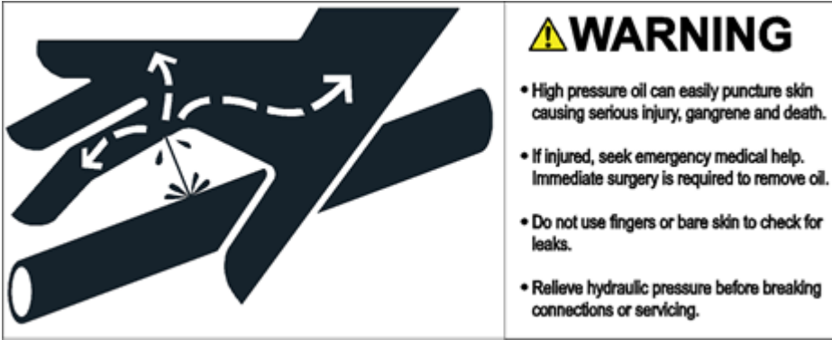
Figure 2.1 – Equipment may contain fluid under high pressure. In event of leakage, jets can penetrate skin and cause severe injury.
