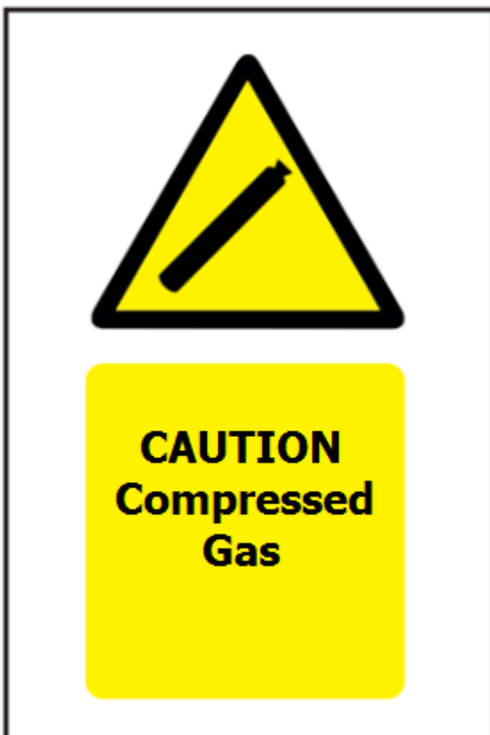
Figure 2.3 – Equipment with accumulators contain gas (nitrogen) under pressure. Can cause explosion hazard in event of fire.
