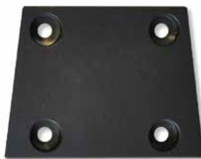
The same plate, with running-in film applied
